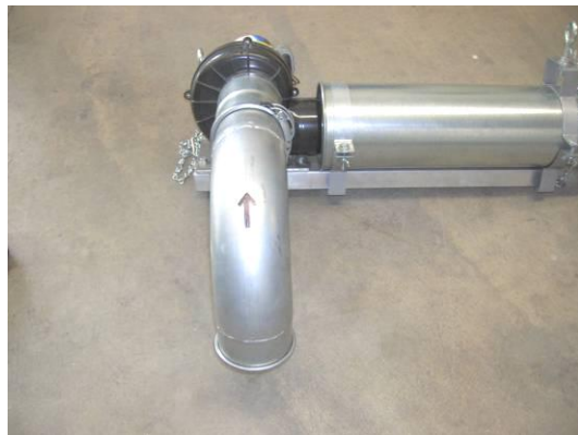
Photo 10: Right angle elbow attached
