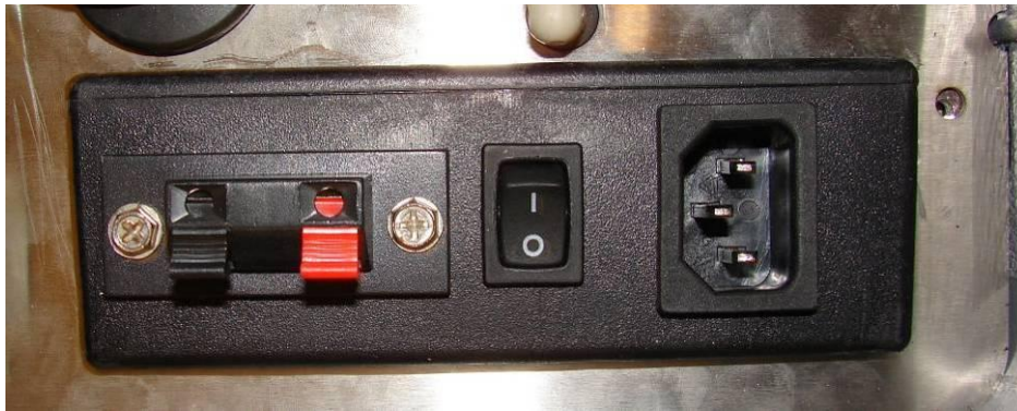
Photo 24: PEMS sensor box power supply with DC and AC power terminals
