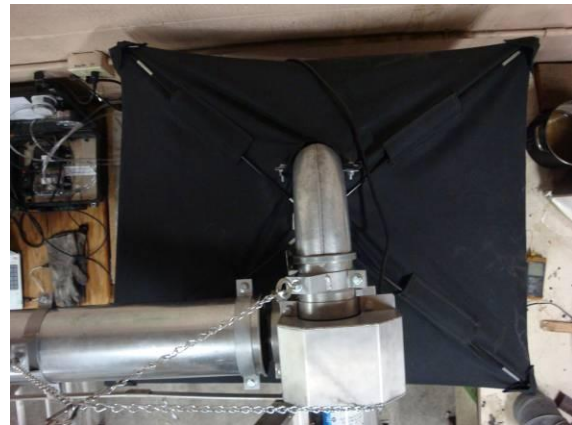
Photo 16: Top view of canopy properly oriented with tent poles inserted
