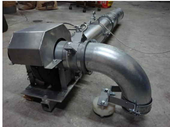
Photo 12: Canopy bracket attached to elbow
