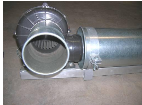
Photo 6: Blower properly aligned with duct
