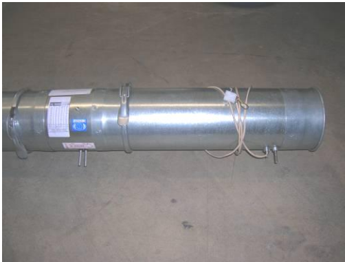
Photo 9: Sampling conduit attached
