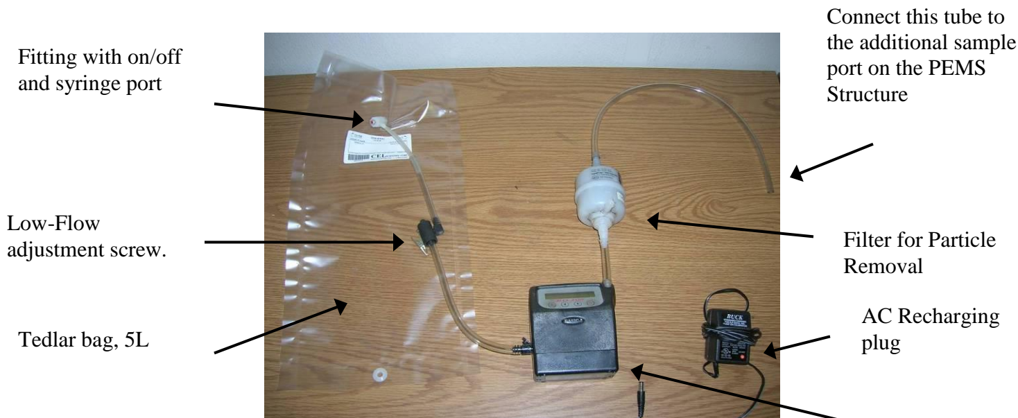
Photo 29: Gas sampling system
