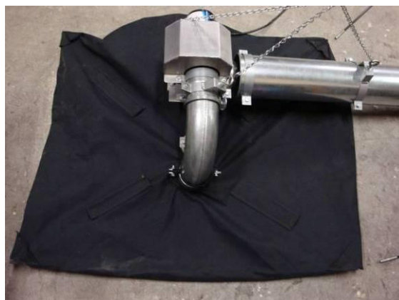
Photo 14: Proper orientation of canopy and canopy bracket
