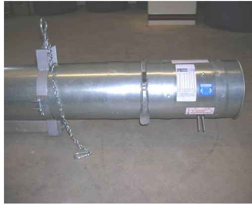
Photo 8: Flow grid section attached with sample ports and flow direction oriented correctly
